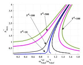
Fig. 5. Comparison of the nonlinear frequency's response for E-E beam A with  $\chi = 0.4$  for different values of F<sup>d</sup>
