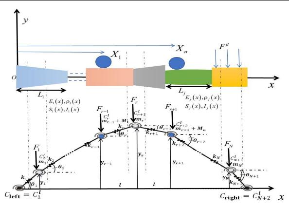
Fig. 1. Typical SAFGB and the corresponding discrete model containing various point masses and subjected to a distributed force
