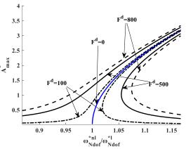
Fig. 9. Comparison of nonlinear frequency response for E-E beam, with  $\beta_2 = 0.25$  and for different values of F<sup>d</sup>
