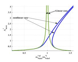
Fig. 4. Linear and nonlinear frequency response for E-E beam A with  $\chi = 0.4$  and F<sup>d</sup>=100
