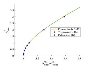
Fig. 2-b. Comparison of the backbone curves for S-S beam B with the results published in [14] for  $\chi = 0.4$
