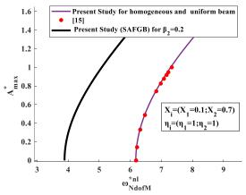
Fig. 13. The effect of the Number of point masses and the nature of beam on nonlinear frequency response for S-S boundary condition
