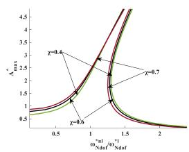
Fig. 7. Nonlinear frequency response for E-E Beam B for different values of  $\chi$  and for F<sup>d</sup>=800
