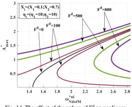
Fig. 14. The effect of the values of F<sup>d</sup> on nonlinear frequency response for S-S boundary condition
