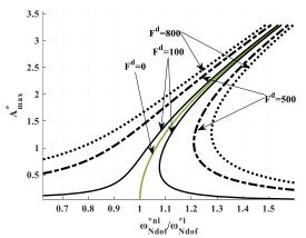
Fig. 10. Comparison of nonlinear frequency response for S-S beam, for  $\beta_2 = 0.25$  and for different values of F<sup>d</sup>
