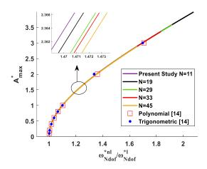
Fig. 2-a. Comparison of the backbone curves for S-S beam A with the results published in [14] for  $\chi = 0.4$
