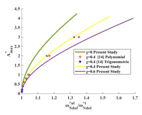
Fig. 3. Comparison of the backbone curves for E-E beam A with the results published in [14] for various values of  $\chi$
