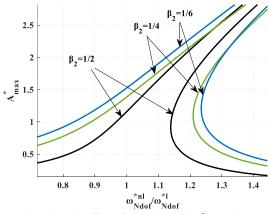
Fig. 11. The effect of the change in  $\beta_2$  on the frequency response for S-S boundary condition and for F<sup>d</sup>=500
